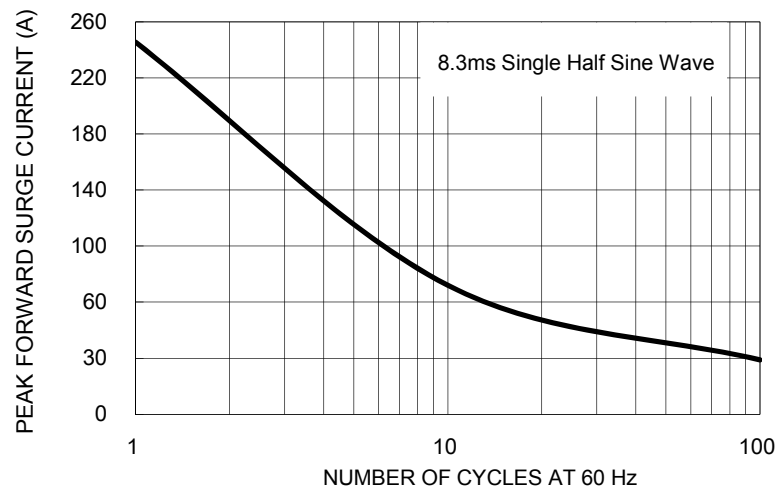
FIG. 3-MAXIMUM NON-REPETITIVE PEAK FORWARD SURGE CURRENT
